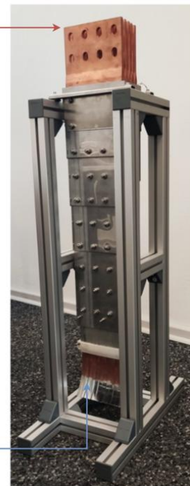
Figure 8 Left: overview of a gas-cooled current lead for 20 kA. Right: tap-off box for the outfeed.
