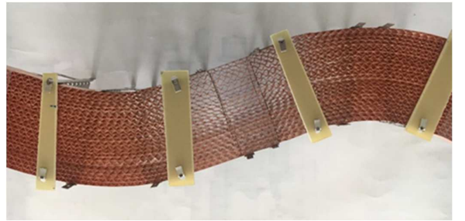
Fig. 2: Stack of 23 superconducting tapes in wave form (overdrawn) with undulated copper tapes as distance holders.
