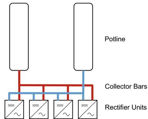
Fig. 2 Collector bars between rectifiers and potline. (Color figure online)
