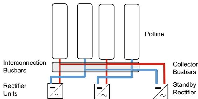
**Fig. 3** Interconnection busbars connecting two potrooms as well as an additional standby rectifier. (Color figure online)
