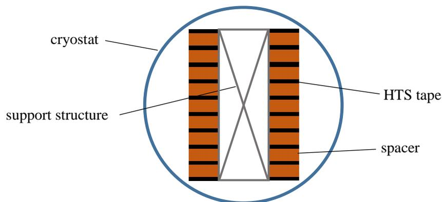
**Figure 4: HTS tape arrangement**
