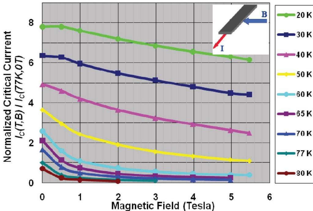
Figure 5: Lift factor of AMSC tape (Performance data courtesy Railway Technical Research Institute, Tokyo, Japan)
