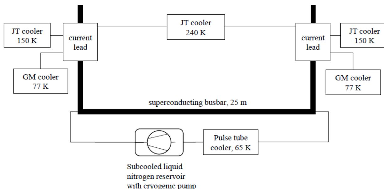
Figure 1 Schematic diagram of demonstrator
